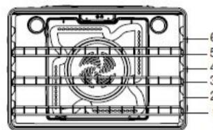
To move a rack, pull it out to the stop position, raise the front edge, and then lift it out. Use the following illustration as a guide for positioning racks.
