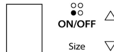
Press ON/OFF to activate the desired cooking element. Press up and down arrow keys to set desired temperature.
