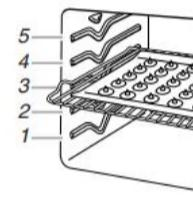
To position a rack, pull it out to the stop position, raise the front edge, and then lift out. Use the following illustration as a guide.
